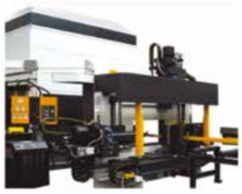
Beam drilling and sawing machines
